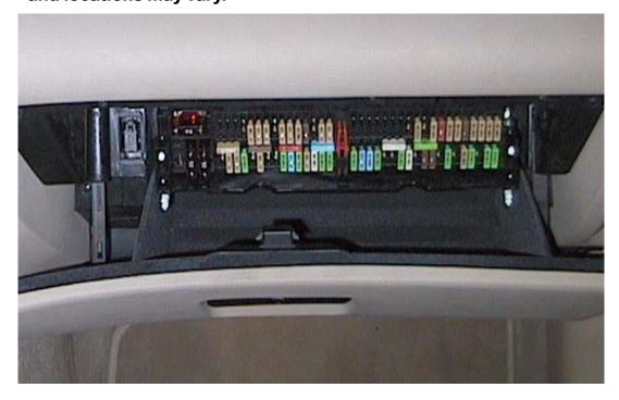
Located above the fuse panel, there are additional high amperage power distribution fuses (F101-F107).
